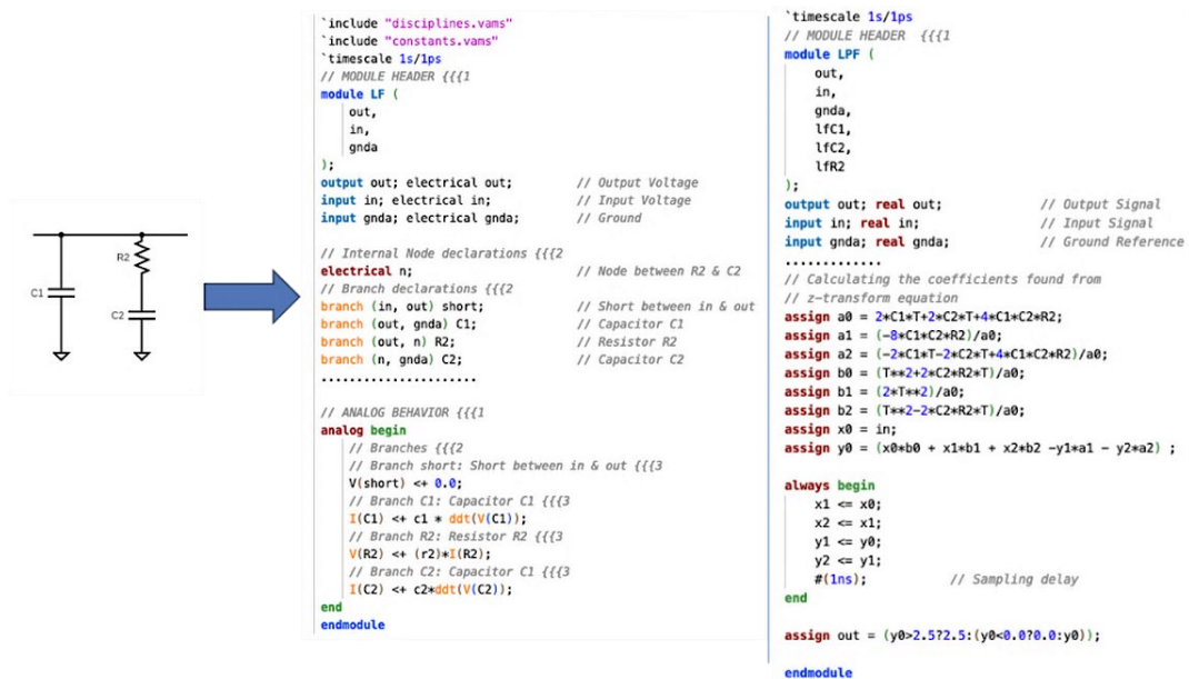
Figure 7. AMS and DMS model of the PLL loop filter
